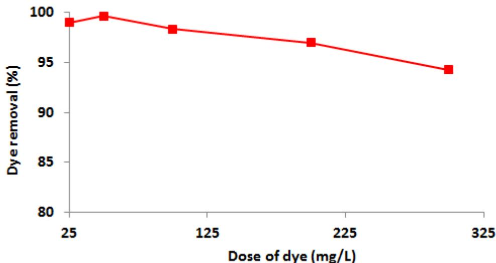
**Fig. 5:** Effect of initial dye concentration on dye removal (current density =62.5 A/m<sup>2</sup>, time =60min, pH=8, conductivity =12mS/cm).
