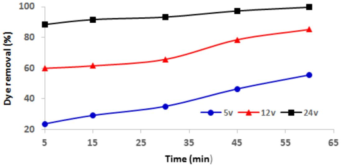
Fig.3: Effect of different voltages on the performance of an EC process (pH= 7, C<sub>0</sub>= 50mg/L, conductivity = 12ms/cm).
