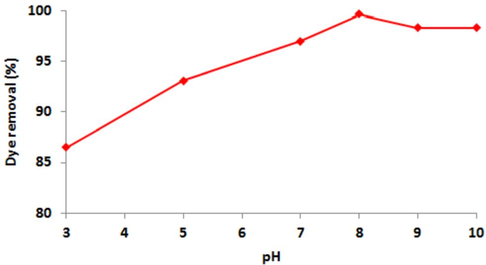
Fig. 4: Effect of initial pH on dye removal (C<sub>0</sub>=50 mg/L, current density 62.5 A/m<sup>2</sup>, time =60min, conductivity =12mS/cm).
